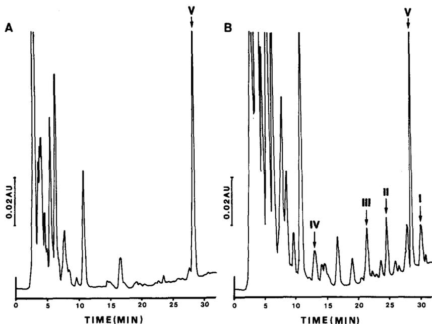
Fig. 4. Typical chromatograms of (A) blank human urine and (B) human urine spiked with I (17.2 nmol/ml), II (34.0 nmol/ml), III (32.6 nmol/ml) and IV (38.0 nmol/ml).
